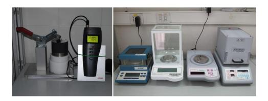
Figure 17. Rotronic instrument, balances and thermobalances in use at BG-SAR (Photos: M. Porceddu).
