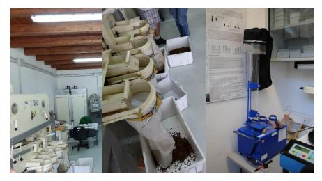
Figure 16. Large mechanical seed separator and small blowing instrument (Photos: D. Ballesteros, M. Porceddu).
